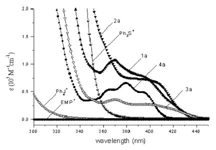
Fig. 1. Optical absorption spectra of onium salts and acylphosphine oxides in CH<sub>2</sub>Cl<sub>2</sub>. (1a, ★; 2a, ▼; 3a, ♦; 4a, ♠; Ph<sub>2</sub>I<sup>+</sup>, ○; EMP, ♠; Ph<sub>3</sub>S<sup>+</sup>, ×).
